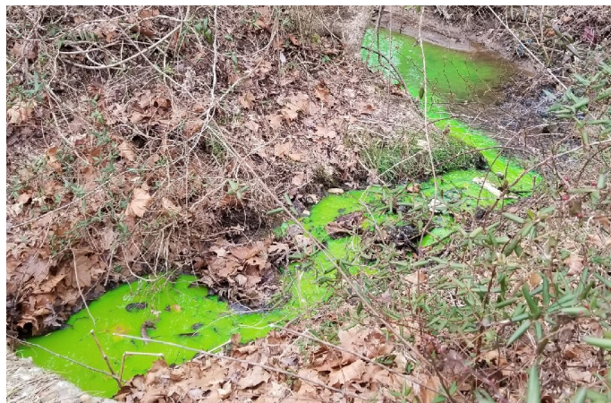
A dye test reveals sewage discharges into a nearby stream. This homeowner was surprised to find they had a straight sewage pipe to a nearby stream, not a septic system.
